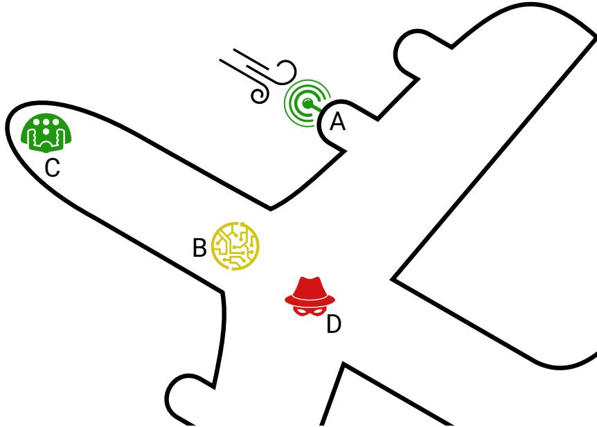
**Fig. 9** The pitot tube indicated by A wants to transmit information to the cockpit and autopilot indicated by C, but lacks the necessary wireless range. It must relay its message through the partially trusted intermediary, B, which is another subsystem of the aircraft.
