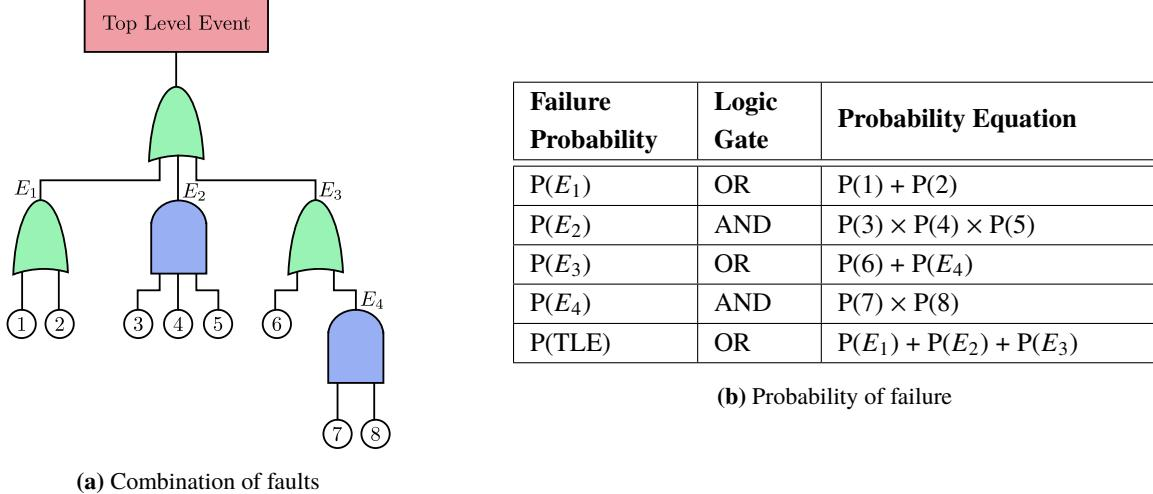
**Fig. 4** A sample fault-tree that uses Boolean logic to combine low level faults (in circles) that lead to an undesired state of a system, i.e. top-level event.
