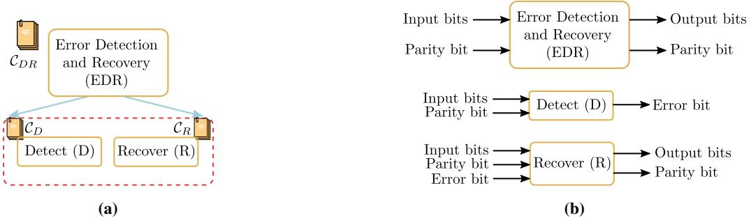
**Fig. 2** (a) Component hierarchy in a Error Detection and Recover (EDR) system composed from components Detect  $D$  and Recover  $R$ . (b) Inputs and outputs for individual components.
