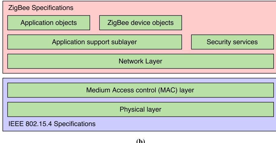
**Fig. 6** (a) Example ZigBee network using a mesh topology showing communication between different nodes. (b) Layered architecture of the ZigBee 802.15.4 protocol stack
