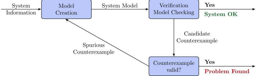
**Fig. 1** Model checking involves entering the system information (as a model) and requirements into a model-checking tool. If there is disagreement between the model’s operation and its requirements, the model checker returns a *counterexample trace*. Otherwise, the system satisfies the specification.
